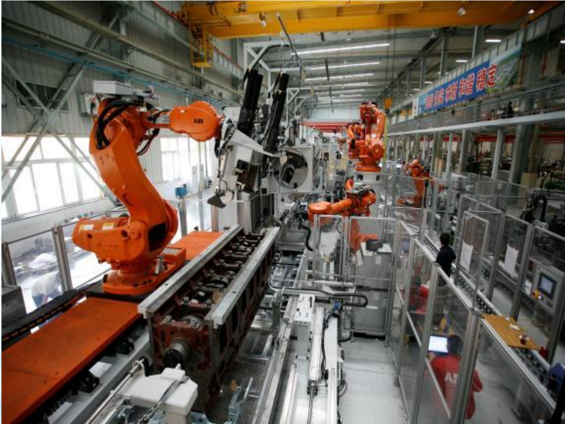
ABB fully automatic engine assembly line
